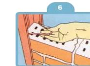
6 Special wire brick ties come with each metal door frame. These ties are for binding the bricks. When mortar is set, remove the spreader bars at base of the metal door frame.
